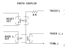
With the external control of the circuit protector, operator can detect a malfunction such as overload or short circuit automatically. Besides, the reset can be performed with external signal that is operator's control system.
